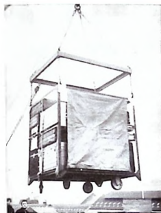
An improved method of handling passenger baggage has been adopted on the Elder Dempster liner "Aurore" using special baggage "cribs" with three permanent wire mesh sides and one adjustable canvas side to permit loading of baggage. A tow bar allows individual hand steering or the cribs can be made into trains of six for mechanised towing. As well as providing greater protection from damage caused by handling, the new system will speed up the discharge of baggage, facilitating customs formalities and enabling passengers to complete landing arrangements in a shorter time.
