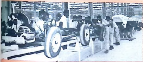
PICTURES . . . how a Volkswagen is made. Engines, axles, gearboxes and chassis are united and then BELOW the body is gently lowered by crane. After the interior and exterior are attached, the vehicle is ready for testing ( BOTTOM ).
