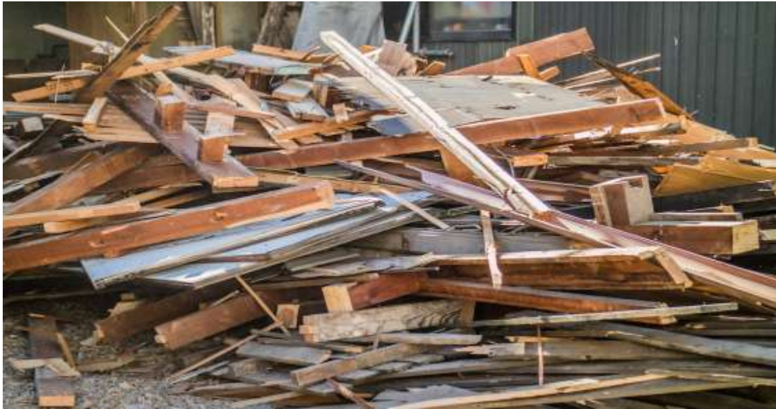
Figure 2: formwork waste (source: Adebayo et al., 2017)
