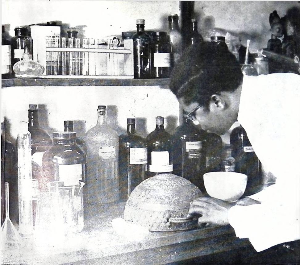
Bronze object being examined after consolidation in a chemical laboratory
