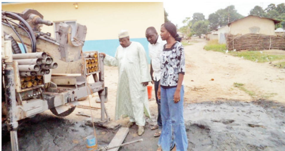
Inspection of the drilling operation at Kudu, Mokwa Local Government where dark shales recovered. These are the envisaged petroleum source rocks.
