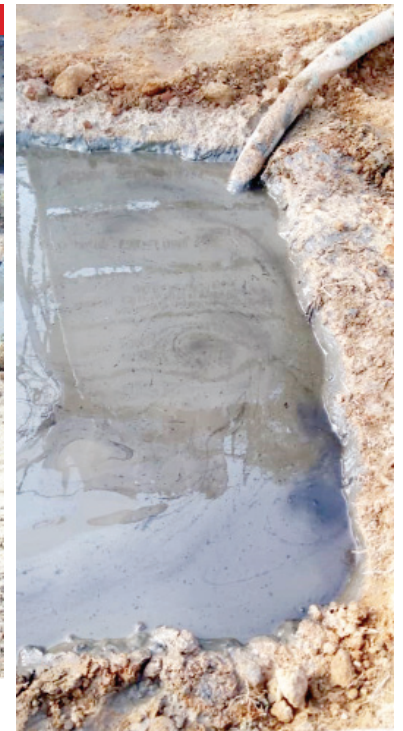
Like at Kudu and Makera, oil slicks (oil shows) oozed out in abundance when the rig penetrates the carbonaceous dark shales
