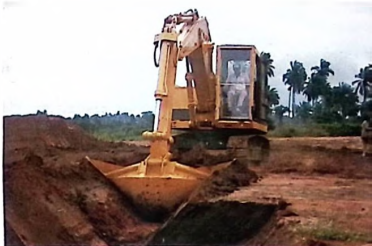
Versatile Cat Hydraulic Excavators, like this 225 with a trapezoidal bucket, dig and maintain irrigation and drainage ditches.
