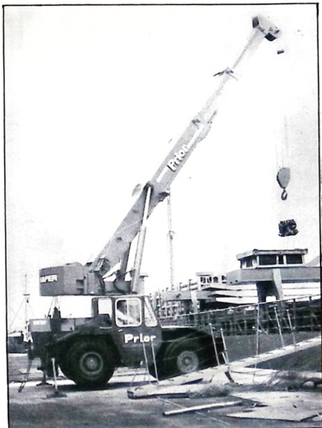
The Rapier HF17 hydraulic mobile crane with maximum capacity of 15 tonnes propped, 8 tonnes free on wheels.
