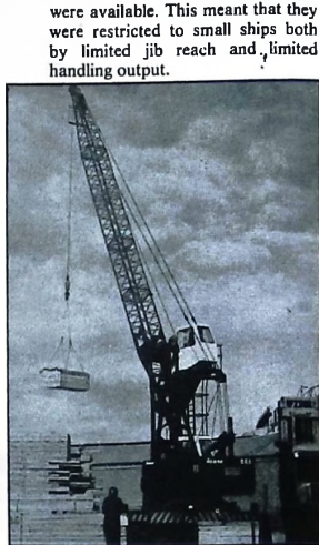
The Jones 565 HLB featuring a high cab and high boom pivot for quayside ship to shore rehandling work.
