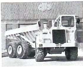
The D330 articulated dump truck with a capacity of 33 tons.
