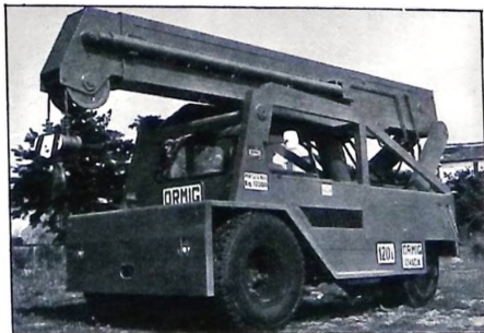
The Ormig 12 tonne telescopic industrial crane with a non-slew boom.
