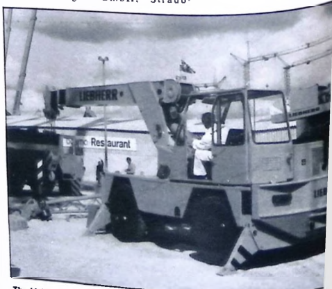
The Liebherr L.1012 12 tonne industrial telescopic crane showing horizontal outriggers.
