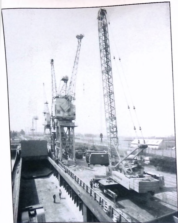
Coles Colossus 4000 handling heavy excavators into barges. This crane also operates with tower and high cab on container handling duties.
