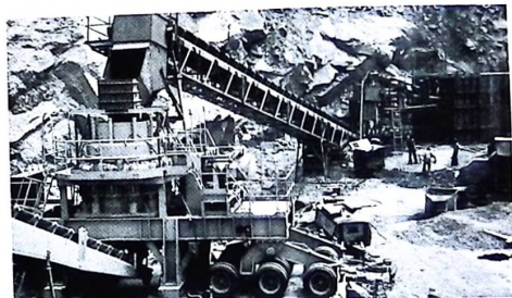
A 5 1/2' mobile Symons cone crusher in a 360 TPH plant in Ore (Nigeria)
