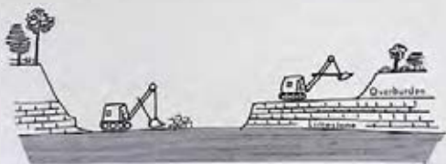
Fig. 98. Excavations removing overburden and limestone rock in a quarry.
