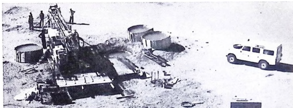
Water-well drilling in Mali, undertaken by the Dutch group IWACO (International Water Supply Consultants). See page 69 for further details.
