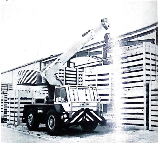
Because of its compact size and rear wheel steer the Jones 1F10 by Jones Cranes is very manoeuvrable and is very versatile in confined spaces.
