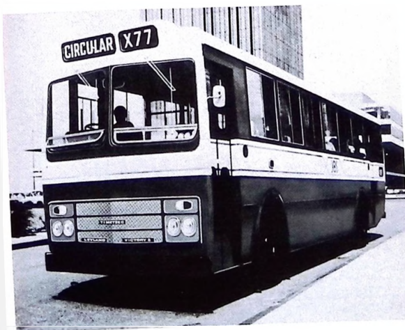
Above, assembly of single-deck bodies in West Africa: where buses have been built in Nigeria, Ghana and Senegal. Below, typical Metsec single-decker in service based on a Leyland Victory 2 chassis.
