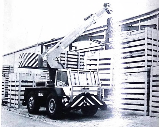
Because of its compact size and rear wheel steer the Jones 1F10 by Jones Crane is very manoeuvrable and is very versatile in confined spaces.
