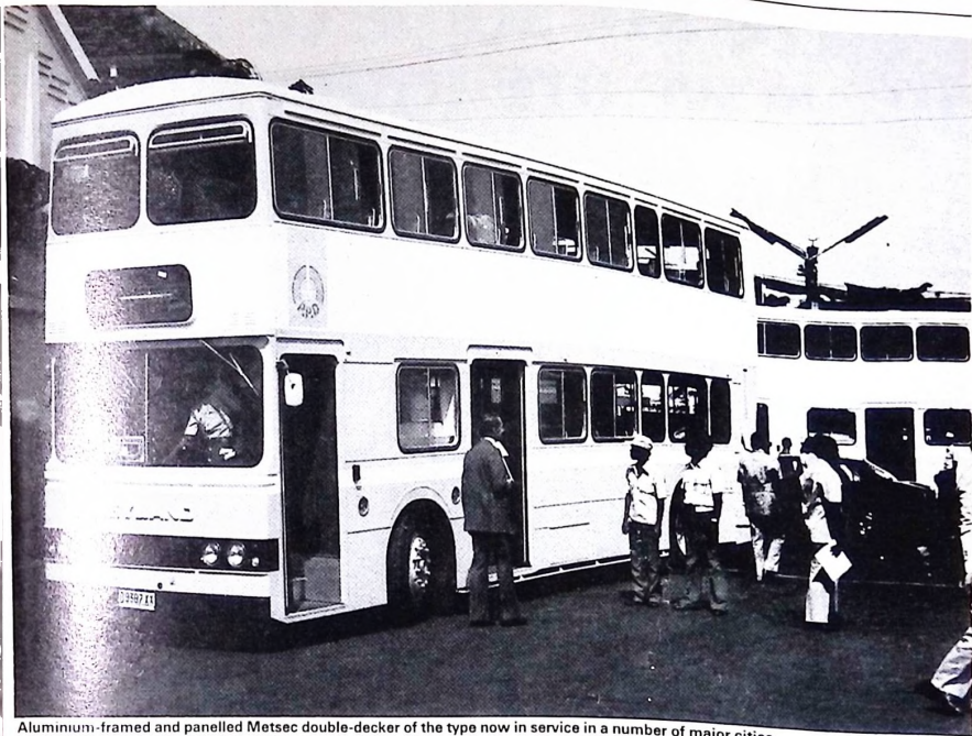
Aluminium-framed and panelled Metsec double-decker of the type now in service in a number of major cities.
