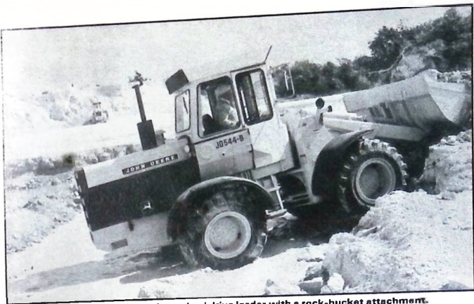
A John Deere JD544B four wheel drive loader with a rock-bucket attachment.
