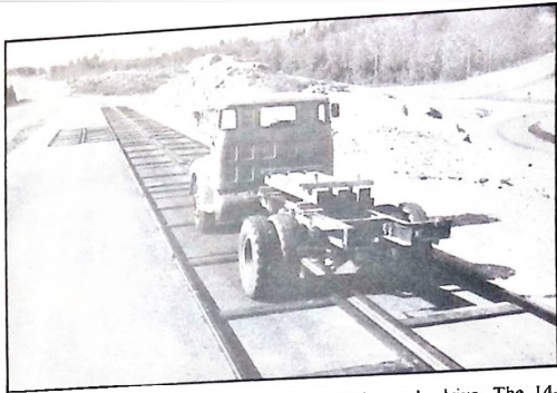
Vibration strip imposes high stresses.
