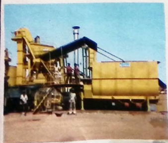
Melting Furnaces for Bitumen
