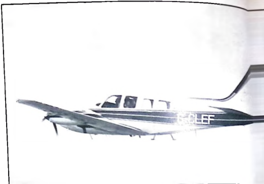
The pressurized Beech Baron 58P is one of the smallest of the light twin-engine offering a pressure cabin for up to six people including the pilot. With six occupants it can fly at 20,000 ft for over 800 nm at a speed of 215 knots (400 km/hr).
