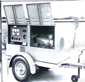
Tropical power - 35kVA air cooled set. 175 power Middle East health clinics.
