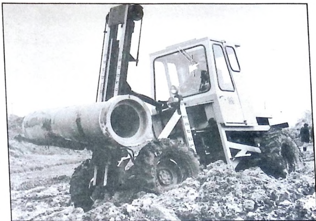
A particular feature of Matbro's M40 centre pivot steer RTFL is its sidelifting mast enabling loads to be lifted vertically, even if the truck is on uneven ground.
