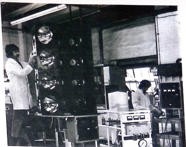
This six direction 300,000 candlea light array is under test, powered by the thermo-mechanical generator. In the white trolley on the right. This converts the propane and electricity, to power the lights and operate the electrical gearless turntable.
