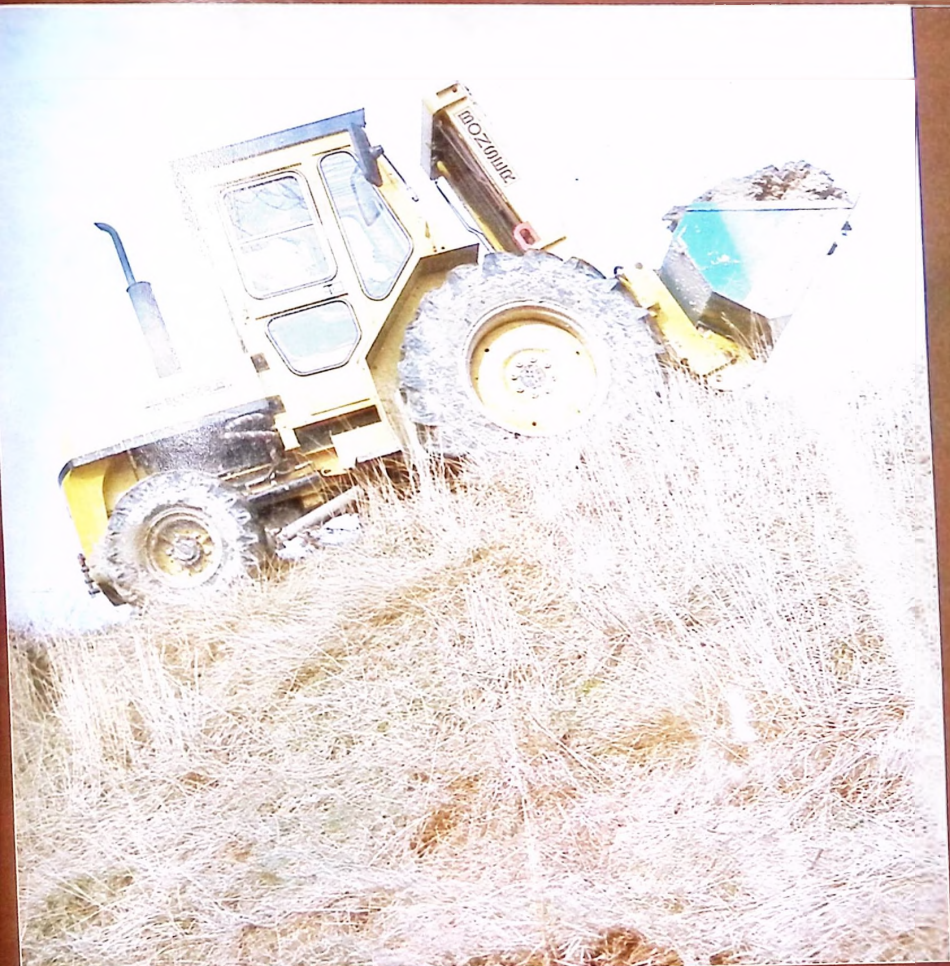
A Bonser RT2500K-4 Rough Terrain Truck with lift capacity of 2,500 kgs.
