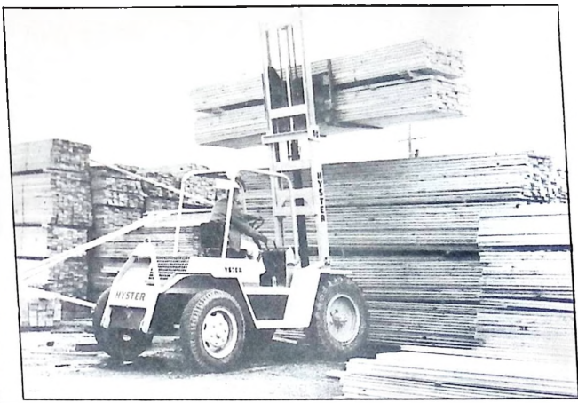
Hyster Pioneer 60 2722 kg capacity lift truck capable of lifting loads of 1.1.3 t to over 9m. Truck is ruggedly designed for use in rough terrain and supply yards.
