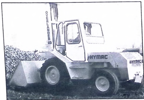
The Hymac Overlander 45 rough terrain fork lift truck. Optional weather proof cab. Fitted with beet bucket.
