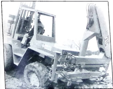
Manitou's 4RM30H is seen here fitted with the PM7002 loader which gives a horizontal lift capacity of 3.5 t at 2 m radius, and 0.80 t at 7.9 m radius.
