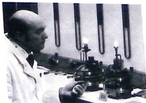
Checking the timing of light flashes from acetylene light units under test at the AGA factory, UK.
