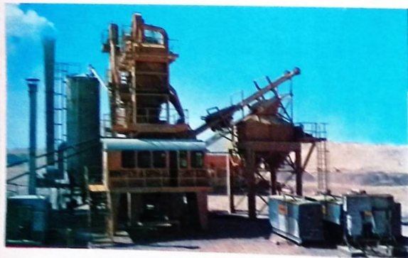
Automatic Asphalt Plants, continuous or batch-type mix, from 12 to 450 Tonn/h.
