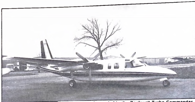
Up to eight passengers and two crew may be carried in the Rockwell Turbo Commander 690B which is powered by two Garrett Aireserch engines of 715 hp each
