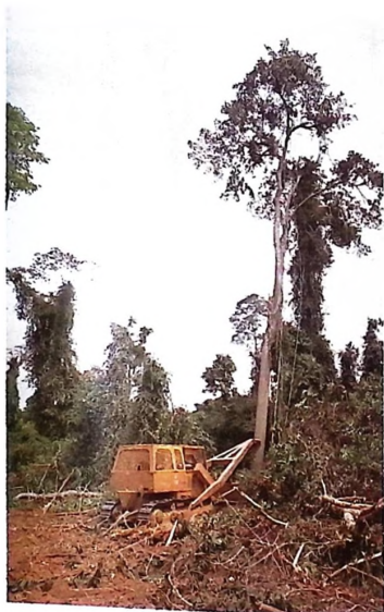
D8K Tractor with Fleco TP8 Tree Pusher, land clearing for Palm Oil Estate Development
