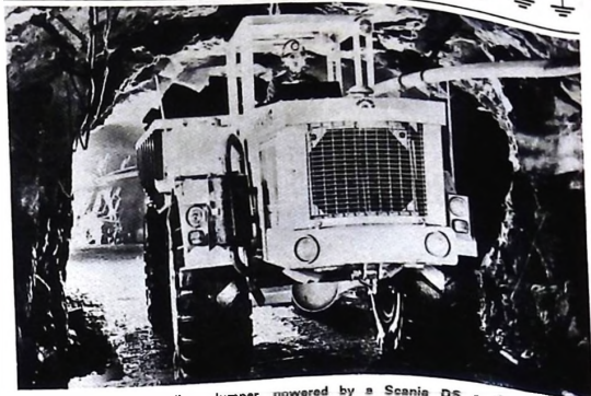
A Kockums 412T medium dumper, powered by a Scania DS engine, working underground.
