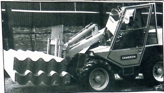
Rated two tons at 20 inch load centres the Sambron J24S can lift up to 20 feet with a towmast.
