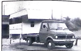
A typical Multicruiser with an accommodation unit jacked off its own pick-up truck.
