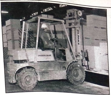
Stacking building boards with a Coventry Climax Universal Major fork lift.
