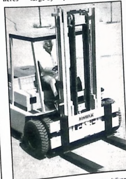
A Bonser D5000K undergoing pre-delivery tests. Exceptional stability and manoeuvrability, together with a number of design innovations are among features Bonser design claim for the new truck which has a lifting capacity of 5000 kg (11,000 lb.) at 600 mm. (24 in.) load centre.
