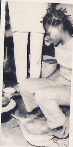
BELLOWS heat the small furnace used to melt down the rare gold.
