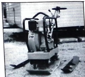
The Weber versatile diesel powered plate compactor for trench work shown on their stand, with plate extension wings
