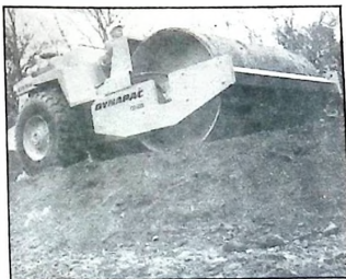
The well proven CA25 to which the new compaction metre can be fitted
