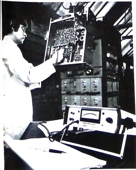
The Racal-Dana wideband millivoltmeter model S301 for the accurate true r.m.s. measurement of r.f., sinusoidal, pulse and noise waveforms.
