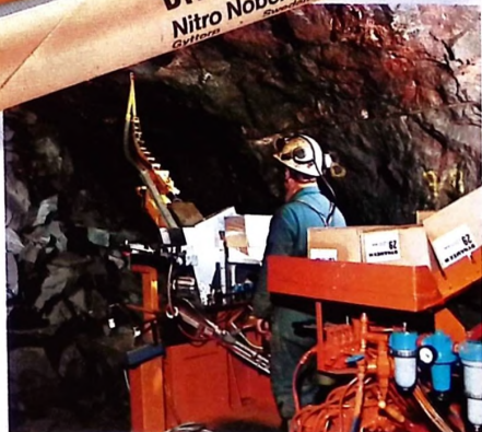
DYNAMEX M in the form of cartridges is adapted for pneumatic charging, for example by using the automatic HF-51 pneumatic cartridge charger with a robot tamping device.
