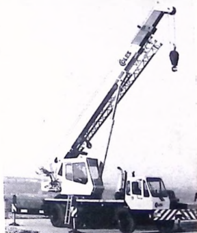
New Coles Supertruck 820 crane with a lifting capacity of 20 tonnes.
