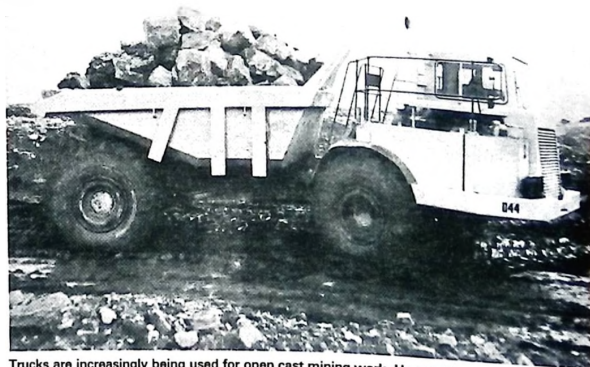
Trucks are increasingly being used for open cast mining work. Here a 40 tonne DJB truck with all wheel drive and articulated frame.
