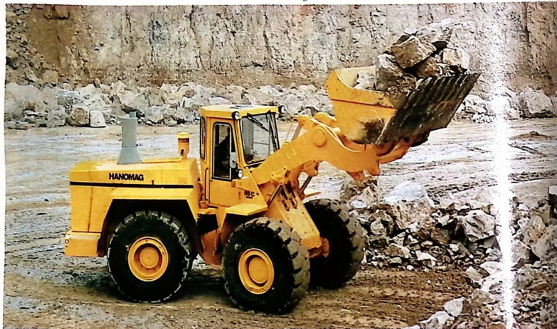
Hanomag wheel loader 66C, turbo-charged engine, 210 hp SAE net.
