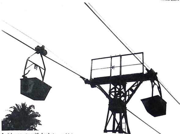
Aerial ropeway with buckets — widely used in West Africa, here at the Ashanti gold mine, Ghana.
