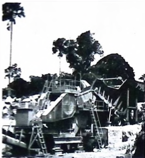
A 100 TPH mobile primary jaw crusher (1080 m wide) in The Ivory Coast
