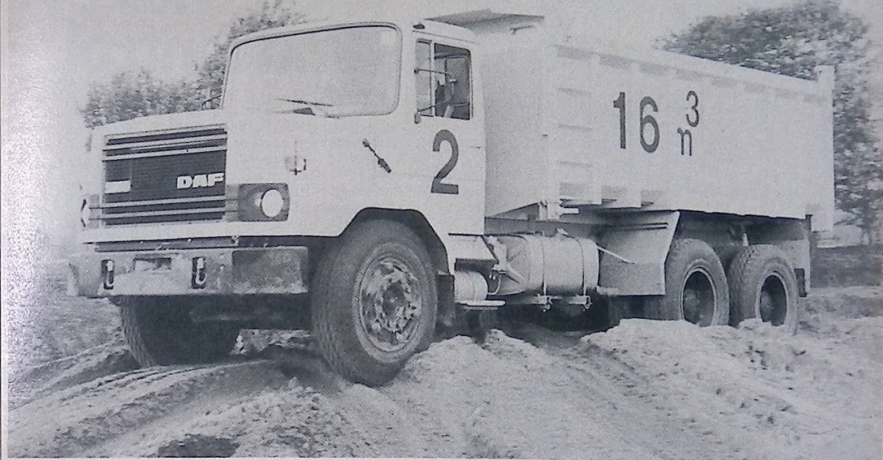
In 5.7m-wheelbase form the N2800 is intended primarily for tipper/dumptruck duties.
