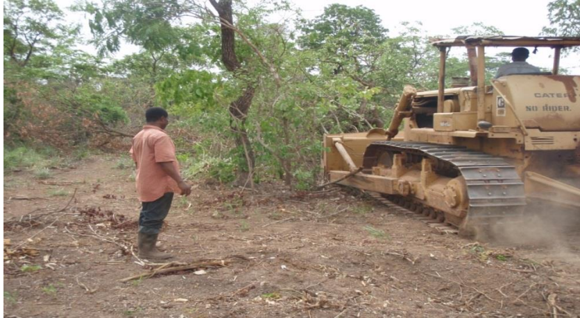
Figure 1: Crawler tractor bulldozer in agricultural bush clearing operation under supervision (Adama, 2013)
