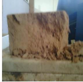
Figure 3: Failure at Maximum Load
