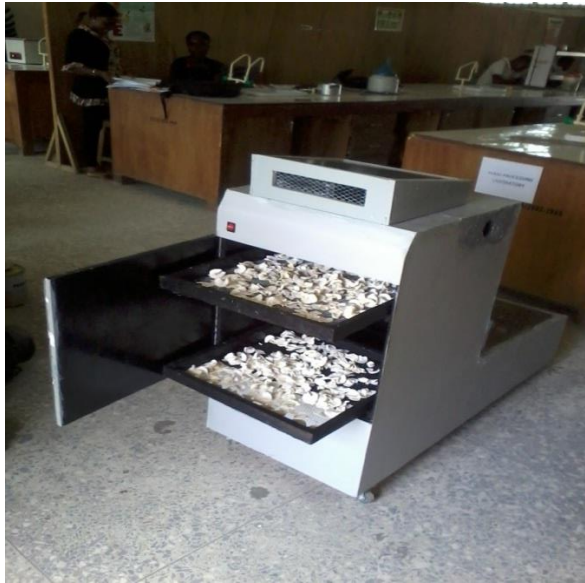
Figure 2: Internal Features Showing the Dried Cassava Chips.
