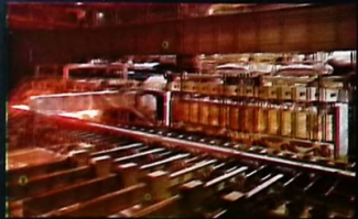
STAHLWERKE PEINE SALZGITTER A.G. Salzgitter, WEST GERMANY Pusher-type 300 t/h capacity each, slab reheating furnaces to feed a 50' hot strip mill
